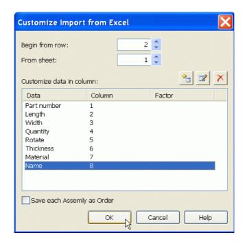
Example 2. Import of a list of parts from an Excel table generated by CADWORK.
